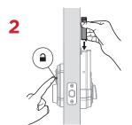
Press and HOLD the Lock button while installing battery pack. Hold button until the latch bolt starts moving on its own.
